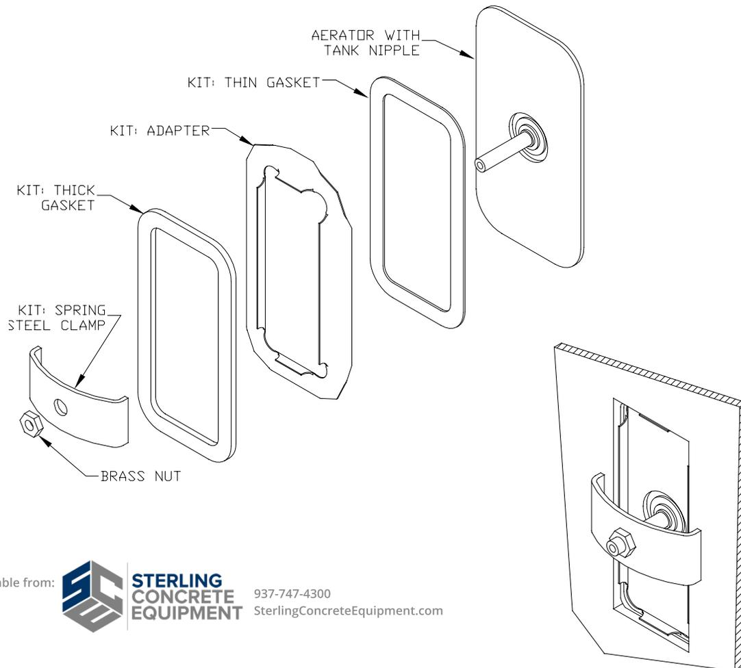
Figure 3: Aerator Kit Installed in Bin Wall
